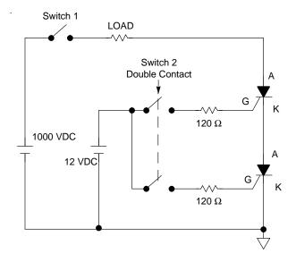
The above diagram can be operated very easily, first, it is needed to close the switch 1 and then, the two SCR can be activated by closing the switch 2; the current value that would be flowing through the SCRs would be the same since the devices are connected in series, nevertheless, the power dissipation in each device could be different since it depends of the Von of each SCR.
