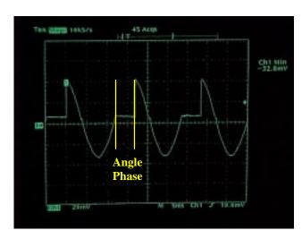
This plot shows how the current waveform looks in the load when it is being controlled the angle phase only in the positive semi-cycle, so in this case it corresponds to the SCR (A).
