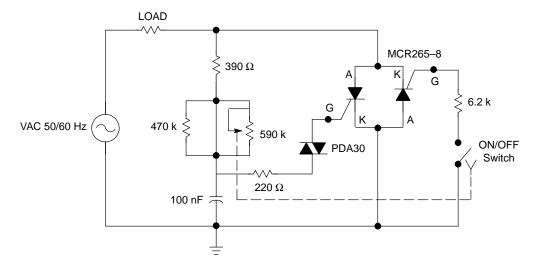
In a different way than in the application note number AND8011/D (High Resolution Digital Dimmer), this circuit is only controlling the angle phase of one half cycle of the ac line which is corresponding to the positive semi–cycle (SCR (A)), therefore, the SCR (B) will be conducting the complete negative semi–cycle of the ac line.
